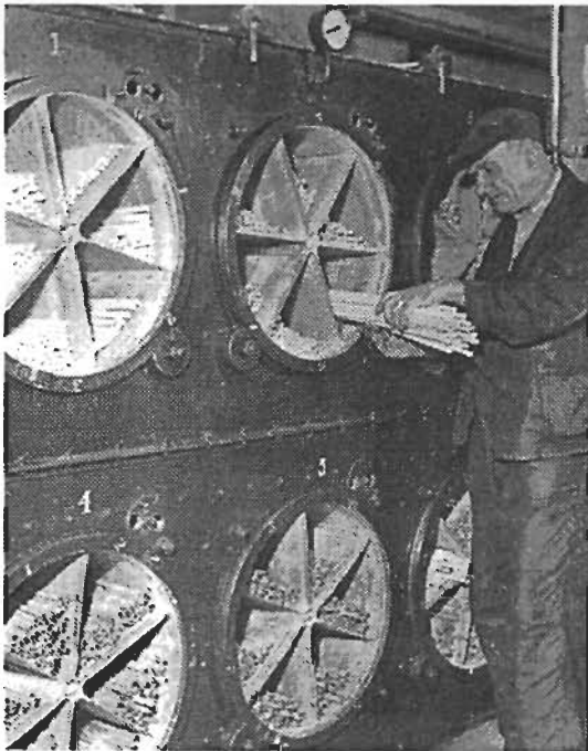
▲ Fig 2 Rotary driers for casein rod, tube and button blanks
