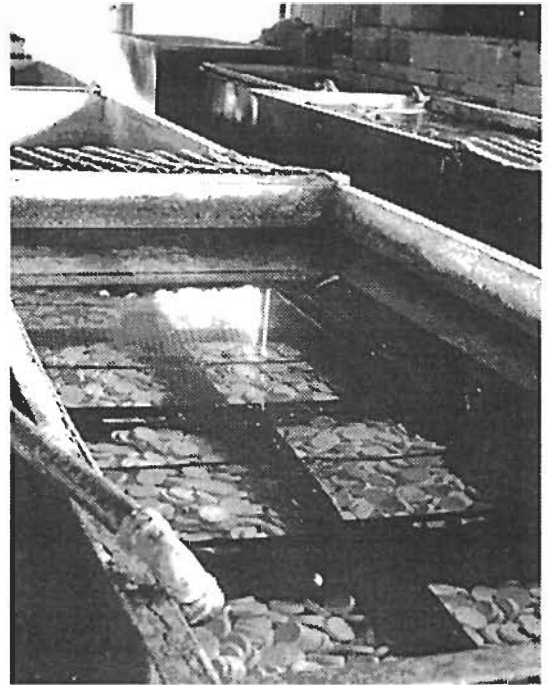
Fig 3 Formalin tanks containing button blanks 1950s
