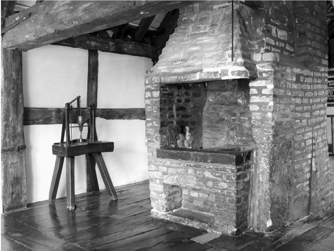
Figure 8 Gloucester Folk Museum top floor chimney adapted to pinhead annealing forge. The machine is a heading ram for attaching separate pinheads.
